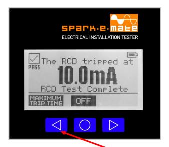
Once the rising fault current test is complete, select maximum trip time to perform 6 tests at 10.5mA at random firing angles. After the six 3003 tripping tests are complete, the results are displayed:
