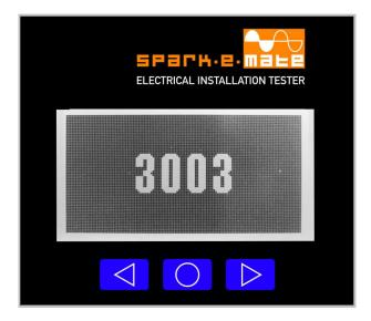
Spark-e-mate applies a slowly rising fault current from 3 -10.5mA until the RCD trips
