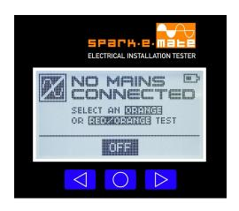
Spark-e-mate running on mains power - ready for RED or RED/ORANGE (a.c.) tests
