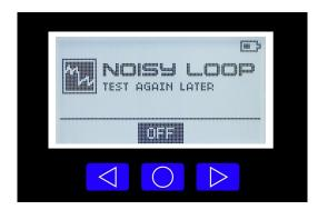
The Earth Continuity test can also be performed more accurately <u>without</u> mains supply however <u>Active</u>, <u>Neutral and Earth must be bridged out at the switchboard otherwise >20 $\Omega$  will be displayed</u>. An easy way is to connect the Active under test to the MEN.
