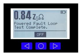
The total fault loop (A to E) impedance reading is then related to the type and rating of the protective devices used to protect the circuit under test, as per AS/NZS 3000 Table 8.1 tested in accordance with Clause 8.3.9.3 (b).
