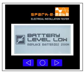
The internal batteries are 6 x AA alkaline. Please note that alkaline or non-rechargeable lithium batteries must be used. Rechargeable batteries <u>cannot</u> be used.
