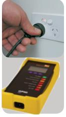
2 Plug into socket outlet or connect active, neutral and earth using the 493L
